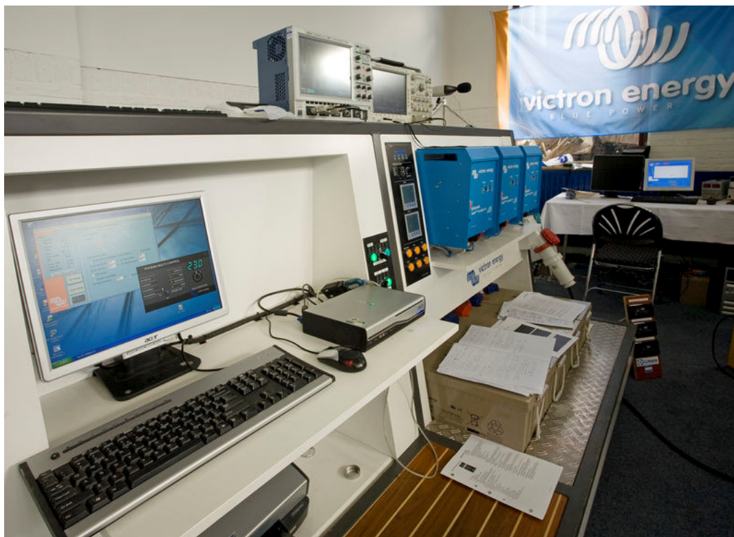
Photo 3: Test bench with three MultiPlus 24/3000/70
